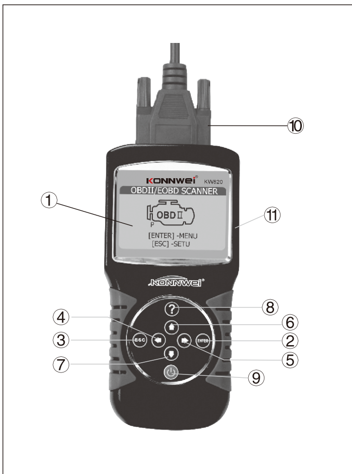
① LCD DISPLAY -- Indicates test results. Backlit, 128 x64 pixel display with contrast adjustment.
